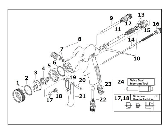
**Note:** Ref. No. 24 (LUNA2-34) is needed for Ref. No. 10 (LUNA2-443) installation. When removing it, be careful not to damage the surface of seat where inserted. A damaged seat may cause air leakage.
